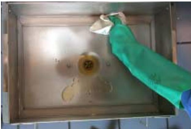
Make sure the inside of the pan is free of all food and breading particles that could prevent the screen from sealing against the bottom of the pan.
