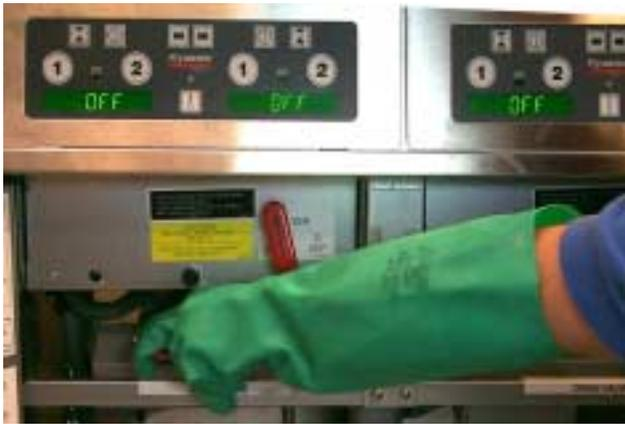
Close the drain-valve and leave the filter pump on to fill the frypot.
