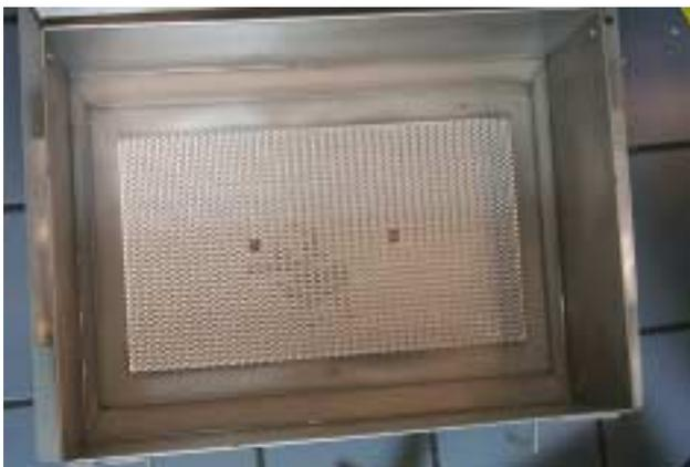
Install the filter screen in the bottom of the pan. Proper operation of the filter system depends upon proper placement of the filter screen. Never filter with the screen alone.
