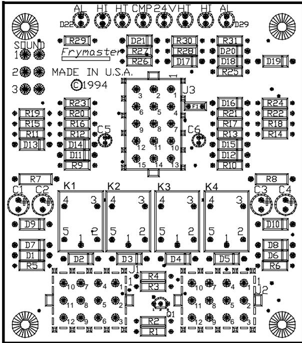
**Note:** The sealed relays are not replaceable. If a relay fails the interface board must be replaced.
