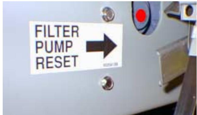
If the pump starts after resetting the thermal overload switch, then something is causing the motor to overheat. A major cause of overheating is when several frypots are filtered sequentially at one time, thus overheating the pump and motor. Allow the pump motor to cool at least 30 minutes before resuming operation.
