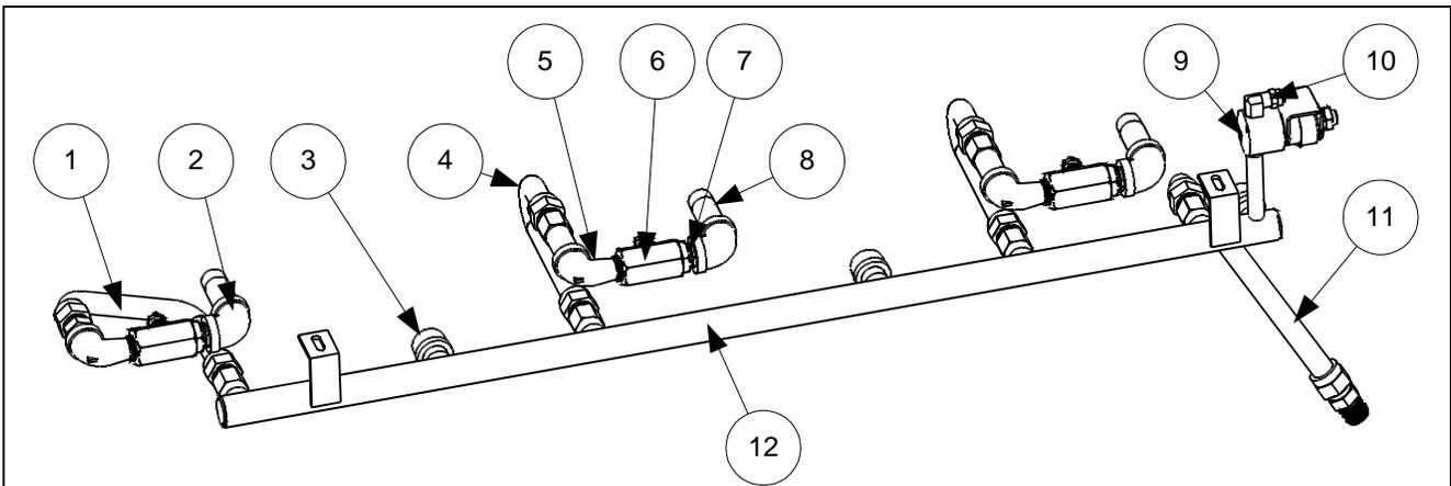
Manifold assembly for all H214, 314 and 414 fryers manufactured after 9/99.
