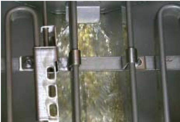
Polishing is a timed process that cleans the oil and washes small particles from the frypot.
