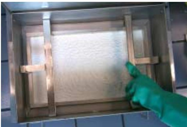
Install hold-down ring over pad, or use ring to push filter paper to the bottom of the pan. Push down firmly to properly seat the paper/pad.
