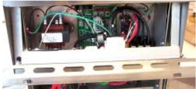
3. Unplug wiring harness at plug on back of controller.
