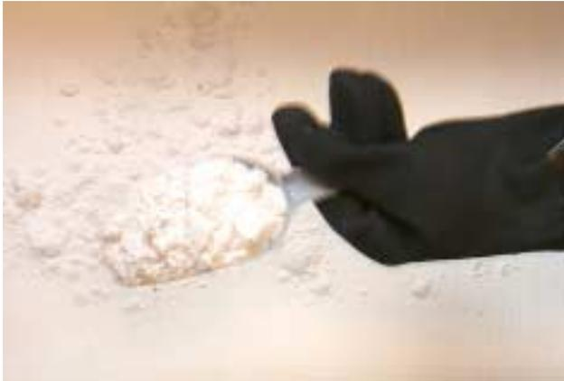
Use 8-ounces of filter powder and spread it evenly over filter paper. **Remember, Do Not Use filter powder on filter pads.**
