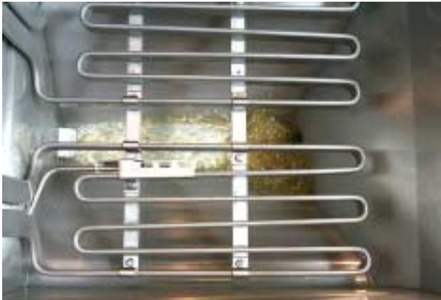
The oil moves through the filter, the frypot and out the open frypot-drain during filtering.
