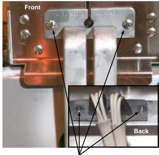
Element-mounting screws and nuts
