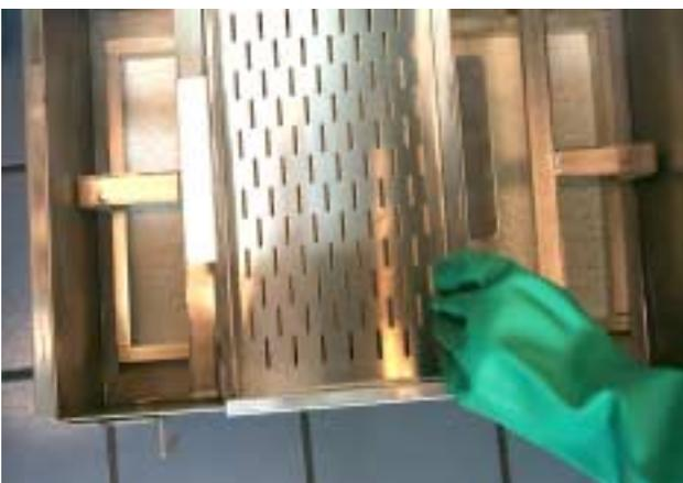
Open the filter-cover, and remove and clean the crumb tray.
