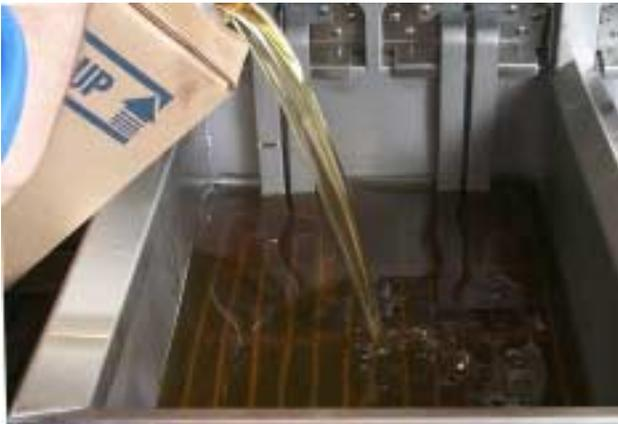
Top up oil level. Some oil may be lost in filtering process.
