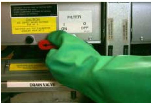
When frypot empties into filter pan, turn return handle to ON. Filter pump will activate.
