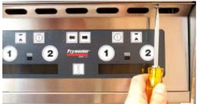
2. Control panel is hinged at the bottom and will swing open from the top.
