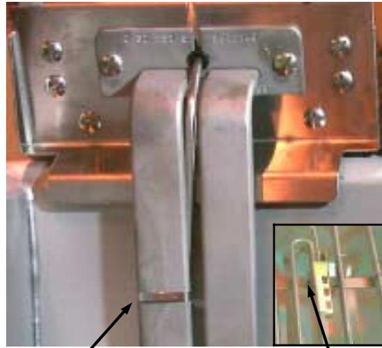
Remove probe clamp (metal Ty-Wrap), and screws securing probe bracket to element
