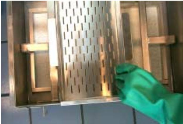
Replace crumb screen inside the filter pan. It's imperative that the crumb screen is installed prior to filtering, for optimum filter-system performance.
