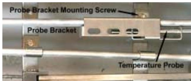
9. Thread the probe wire through the hole in the tilt plate assembly and remove the probe and the securing components from the element.
