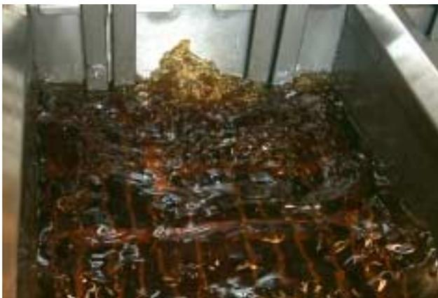
When the filter pan empties, bubbles will form in the frypot. Allow bubbling to continue 15-20 seconds to ensure the oil return lines are clear of shortening.
