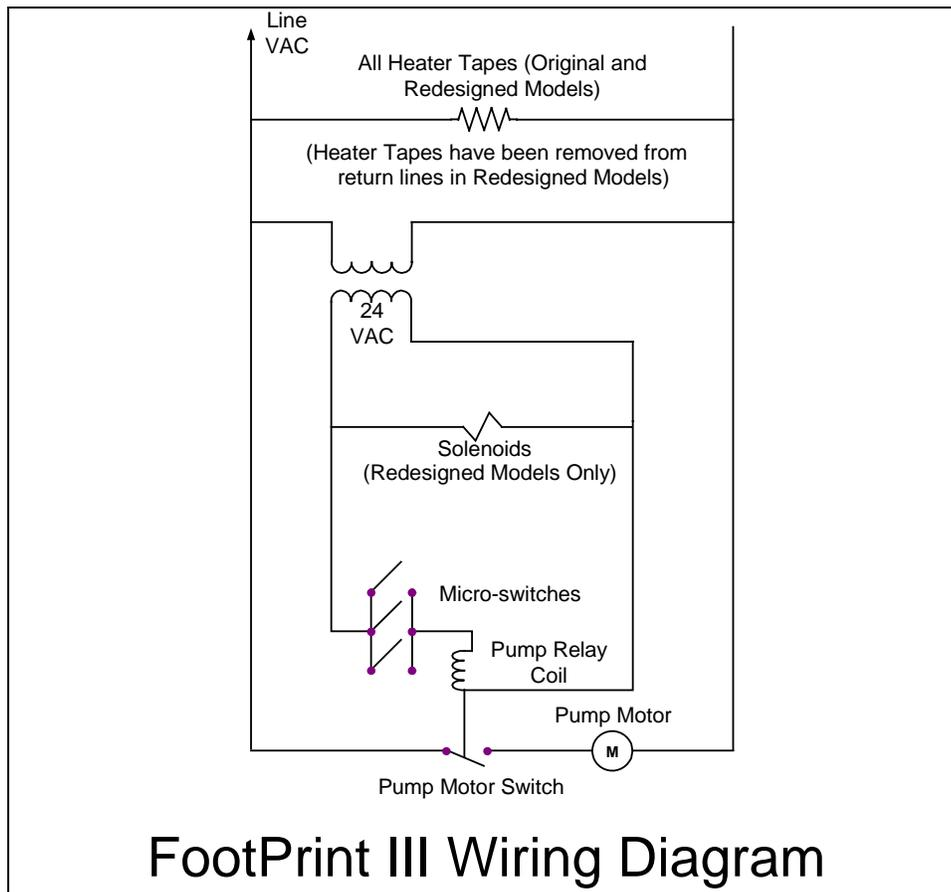
Operation of the redesigned FP-III system is the same as for the original design.
