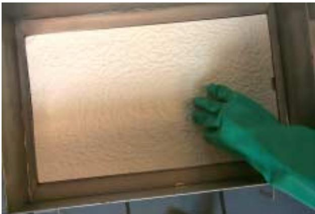
Place pad evenly on filter screen. If paper is used, position the paper on top of the pan with the edges evenly overlapping. **Ensure that the screen is in place prior to pad or paper placement.**
